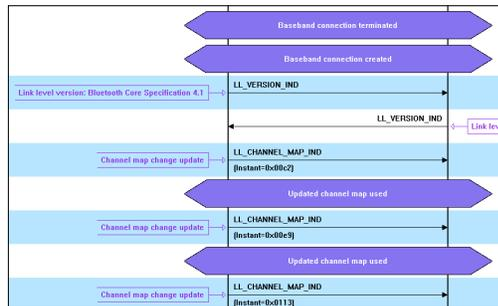
**Message Sequence Charts** tell the complete story of the Bluetooth connection, but in clear and descriptive terms that give the developer a clear linear sense of what actually happens and in what order. This view helps to bring clarity to what can be an otherwise overwhelming flood of granular data.
