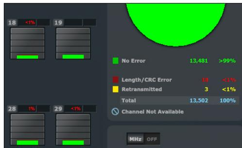
**Packet Error Rate Statistics** help developers ensure that their Bluetooth devices under test are communicating effectively and have sufficient throughput in noisy environments as well as quiet ones, and can even provide indicators of 802.11 coexistence issues.
