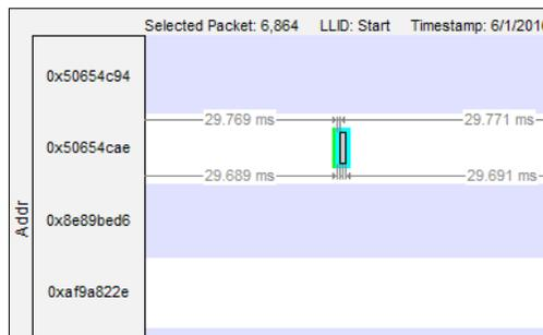
**Bluetooth Timeline** gives the details on packet size, frequency and interframe spacing to help developers resolve issues related to throughput, power consumption and timing that may be adversely impacting Bluetooth data communications.
